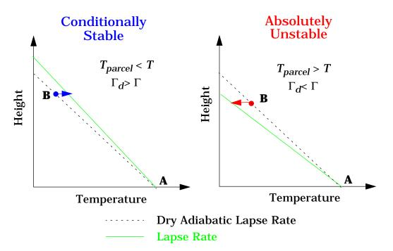
temperature must decrease at the dry adiabatic lapse rate (the dashed line). At some height, **B**, let's compare its temperature,  $T_{parcel}$ , to the air temperature, *T*. The air parcel's temperature is less than the local temperature; thus, it is denser than the surrounding air.
