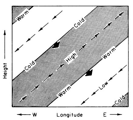
and cold to temperature, the thin arrows show the perturbed wind field, the short thick arrows indicate the wave's phase velocity and the shaded regions show upward motion.
