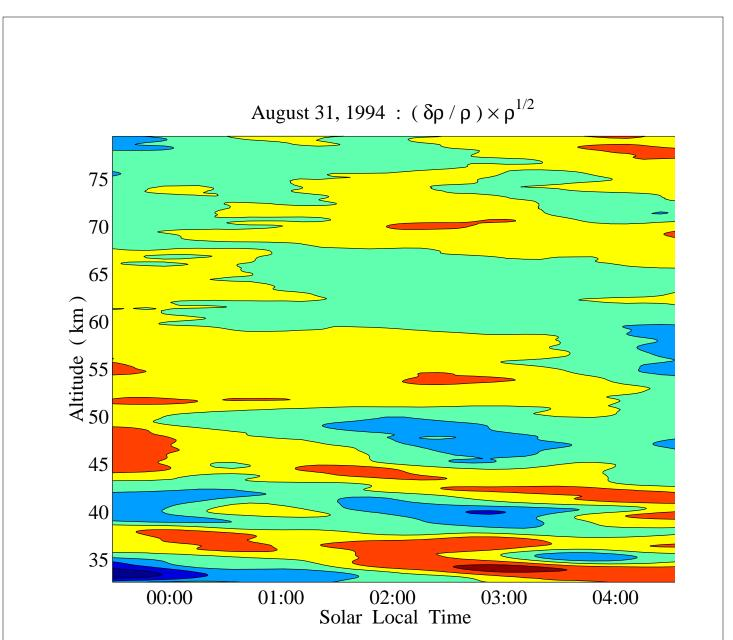
The large-scale wave structures are much clearer when the perturbations are scaled by the square root of the density.
