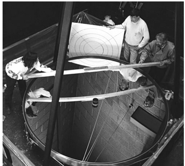
Figure 5. Photograph of the 2.65-m diameter liquid mercury mirror used at the University of Western Ontario’s, Purple Crow lidar. See color insert.
